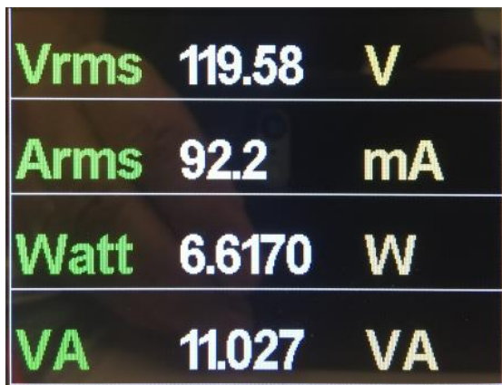
Figure 3: Current, Power and VA drawn from 120Vac outlet
