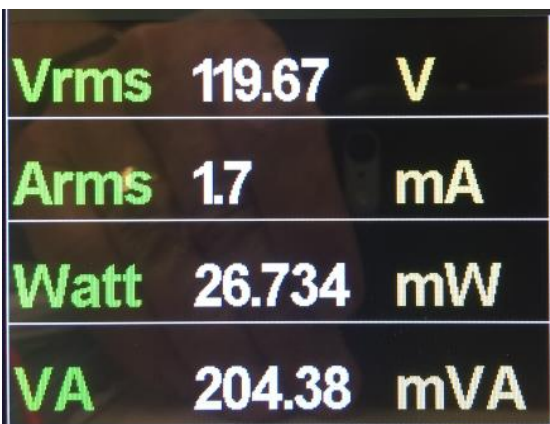
Figure 6: No Load Current, Power and VA drawn from 120Vac outlet
