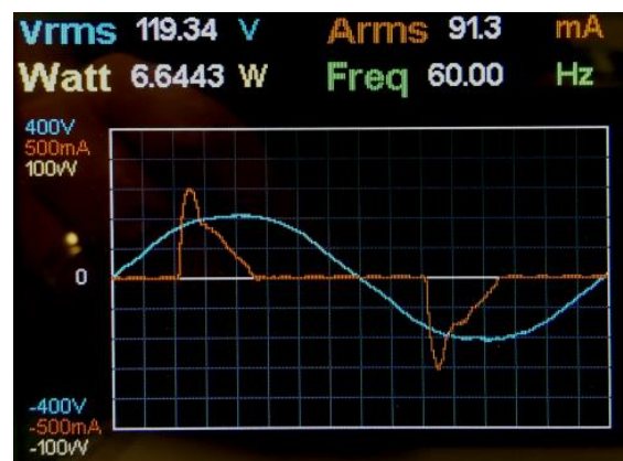
Figure 5: Phone Charger Voltage and Current
