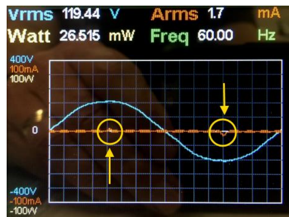
Figure 8: No load Voltage and Current waveform
