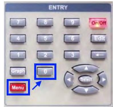
Once in the System Setting menu, press the **Edit** key and use the cursor keys to scroll through the available settings. To change a numeric setting, enter the new value and press the **Select** key inside the cursor keypad. To change alternate fields, use the left and right cursor keys to move between field settings and press **Select** when done.
