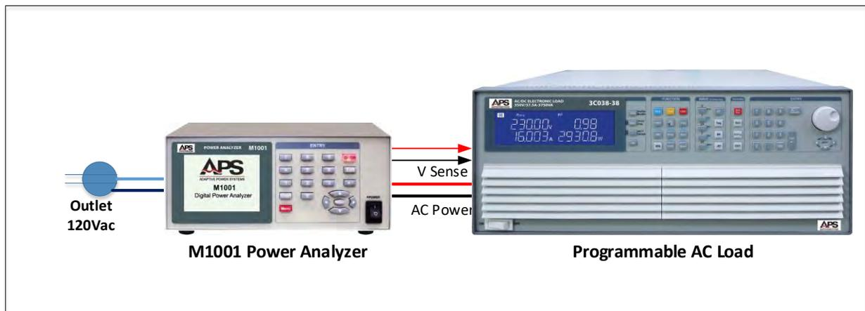
Figure 1: Equipment Setup
