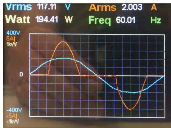
**Note** that the Graph or Scope mode is not that relevant for taking actual measurements but rather serves to be able to identify any anomalies in either voltage or current waveforms. In this example, it is immediately obvious that the load current represents a rectified AC current or a non-linear load, which explains the high level for current distortion. To toggle back to the numeric meter display, press the **Graph** key again.
