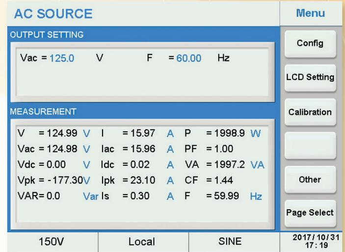
AC Voltage & Frequency Setting and Measurements
