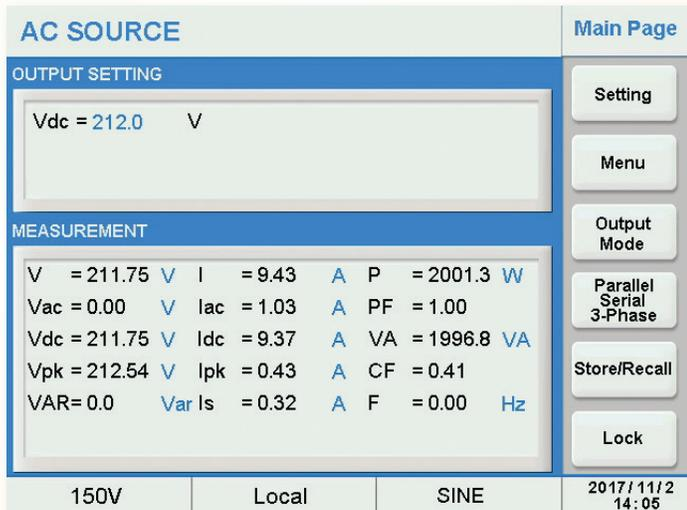
DC Voltage Setting and Measurements
