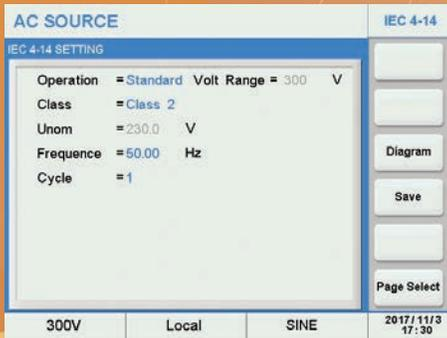
IEC 61000-4-11 Voltage Dip Test Screen - Class 2
