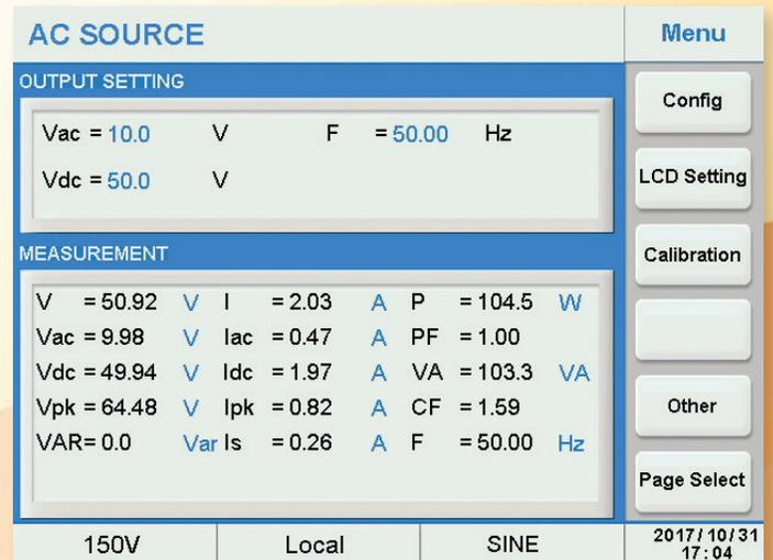
AC+DC Voltage, Frequency Setting and Measurements
