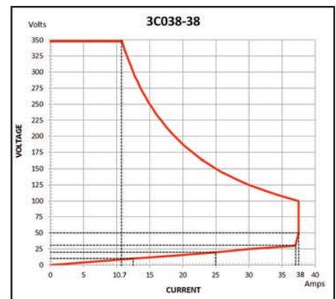
Model 3C038-38 Load Power Curve - 3750W
