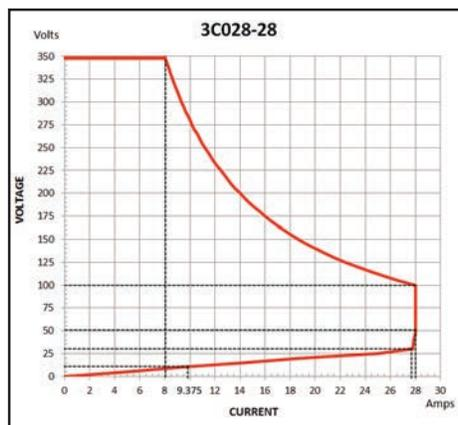
Model 3C028-28 Load Power Curve - 2800W
