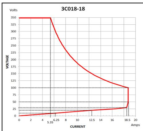
Model 3C018-18 Load Power Curve - 1875W
