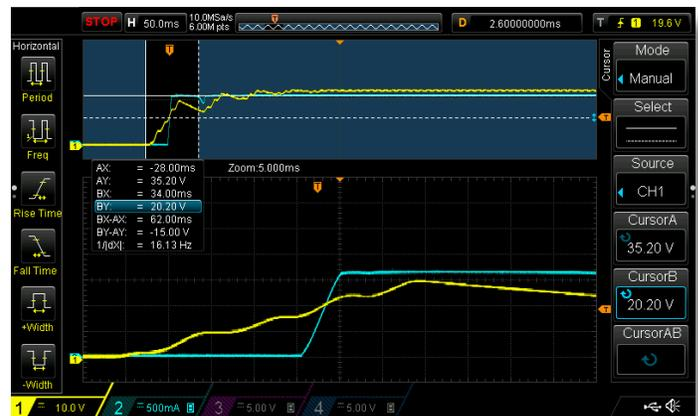
Figure 17: Start-up delayed timebase zoom
