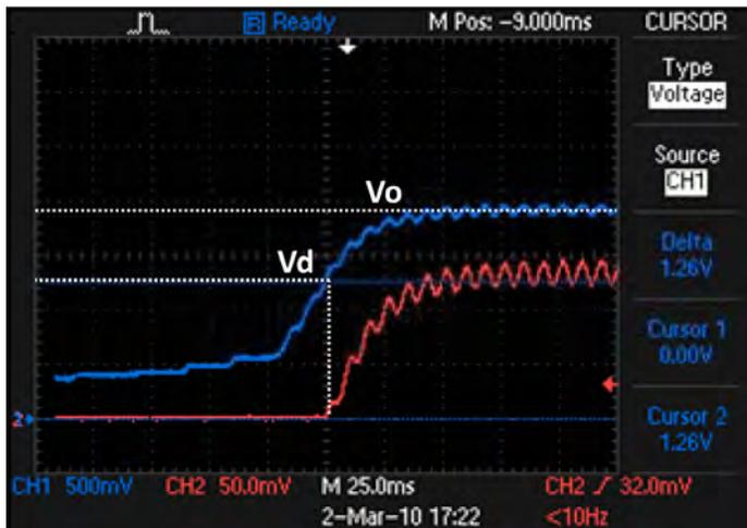
Figure 6: Actual LED load voltage (blue) and current (red)
