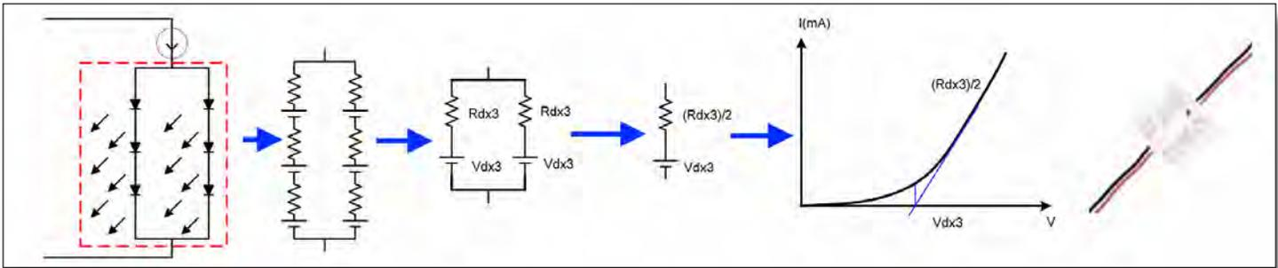
Figure 4: Equivalent LED Parallel/Series Electrical Circuit
