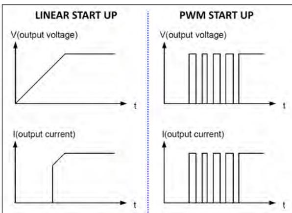
Figure 18: Linear supply versus PWM supply
