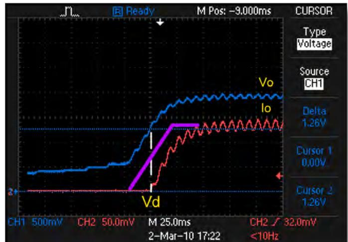
Figure 7: Voltage (blue) and current (red) using CR mode
