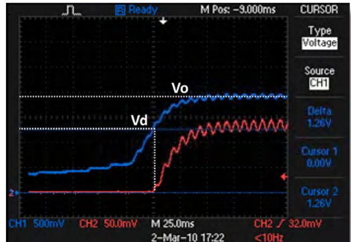
Figure 10: Voltage (blue) and current (red) using LED mode
