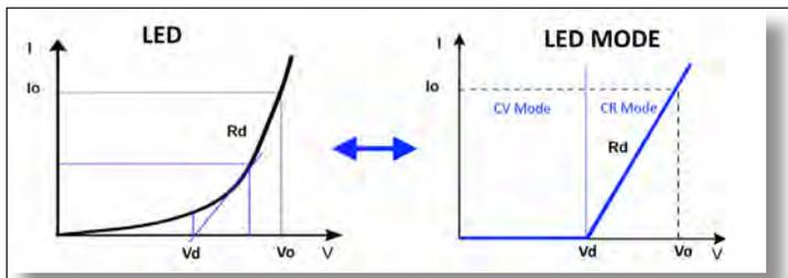
Figure 9: I-V Impedance curve for LED versus electronic DC Load in LED mode
