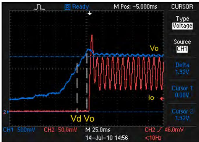
Figure 8: Voltage (blue) and current (red) using CV mode
