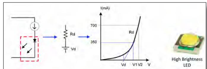
Figure 1: Equivalent LED Electrical Circuit
