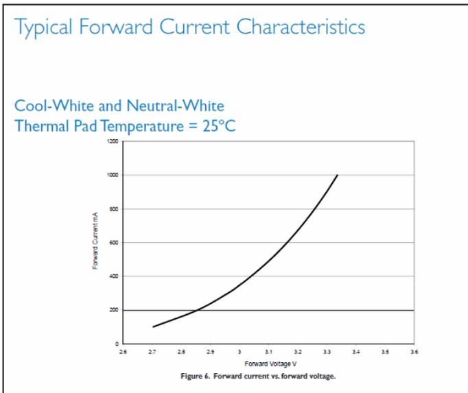
Figure 12: Philips LUXEON Rebel forward voltage chart
