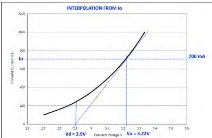
Figure 13: Tangent of forward voltage curve
