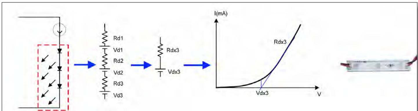
Figure 3: Equivalent LED Series String Electrical Circuit
