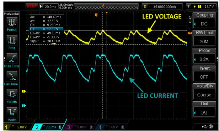
Figure 2: LED driver output voltage and current waveforms
