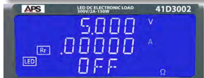
**Note:** Always turn on the LOAD first before you apply input power to the LED driver. Not doing so will result in the driver trying to drive current into an open circuit which means it will most likely not turn on.
