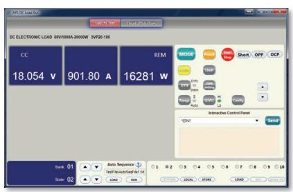
DC Load GUI Main Screen Controlling 5VP Series High Power Load
