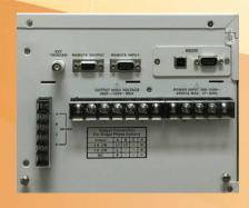
All load connections are made at the rear panel. Both delta and Wye three phase loads are supported using the Phase A, B, C and Neutral terminal posts. Connections for single and split phase or DC loads are indicated on the rear panel as well. A safety cover is provided. For higher power loads, external voltage sense is available to compensate for load wire drops.
