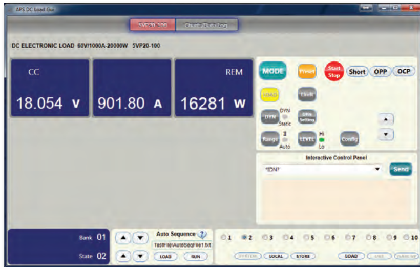
DC Load GUI Main Screen Controlling 5VP Series High Power Load
