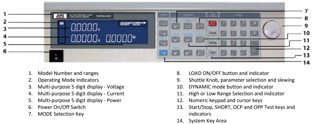
Figure 6-2: Front Panel User Controls and Indicators
