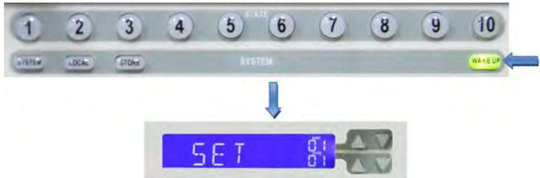
2. Select the memory location (BANK and STATE) that is to be used at power on. Once the correct location has been selected, press the STORE key. The example below shows BANK 01 STATE 01. After pressing the STORE key, the LCD will revert to the normal (Nor) message.
