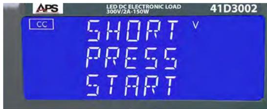
If the input voltage drops below 1.0V, the results will show PASS when the 10 second test interval is completed. If not, the result will be FAIL.
