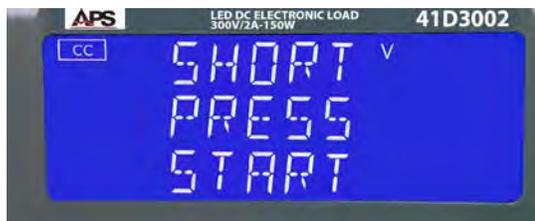
Press the SHORT key again to display the TIME screen. Press UP cursor key or turn the shuttle to select 10000 msec.
