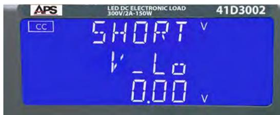
Press START/STOP key to start the short test. The relay should engage shorting the load input terminals.
