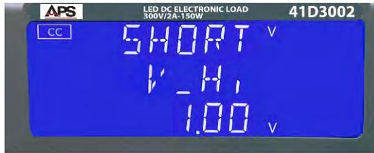
Press the SHORT key again to display the V\_Lo screen. Press DOWN cursor key or turn the shuttle to set 0.00 V.
