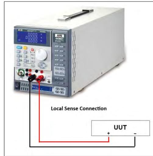
Figure 7-2: DC Load Connection with Internal Voltage Sense
