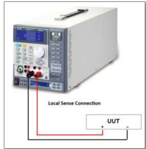
Figure 7-2: DC Load Connection with Internal Voltage Sense
