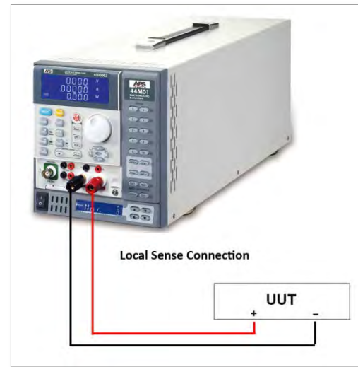
Figure 7-2: DC Load Connection with Internal Voltage Sense
